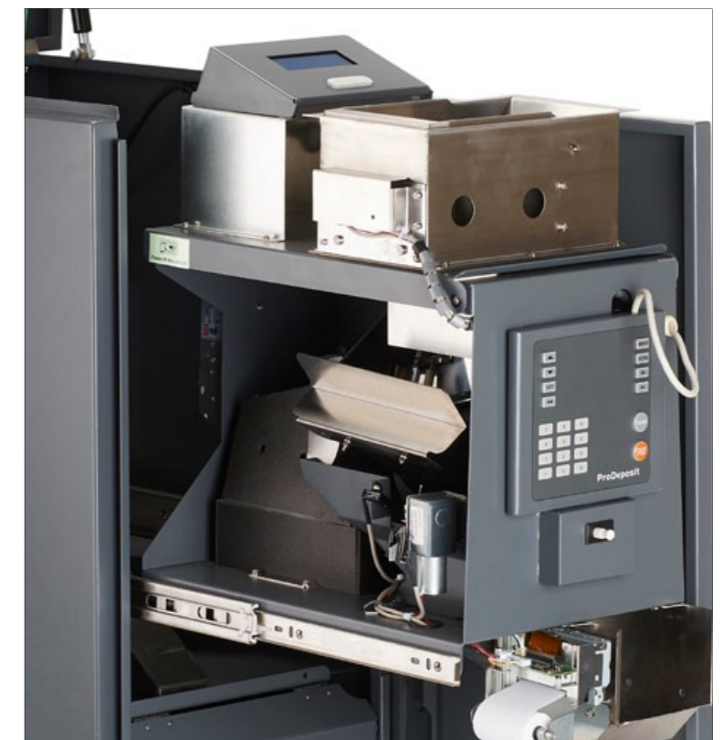
Coin counting unit with overflow protection and motorized cleaning mechanism
